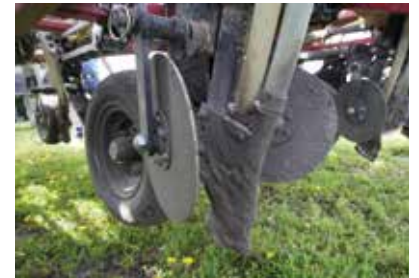
Jonah is running Atom-Jet's 3" paired row openers and row closers for Bourgault Paralink
