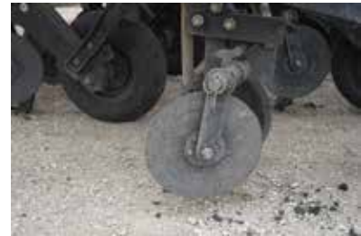
David is running his row closers with single shoot openers on his Bourgault Paralink
