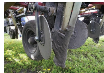
Jonah is running Atom-Jet's 3" paired row openers and row closers for Bourgault Paralink
