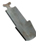
Steel piece welded to front of opener to protect liquid line from trash.
